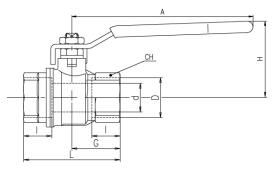
d shows the nominal flow diameter. Actual flow diameter complies with full port DIN 3357 part 4.
