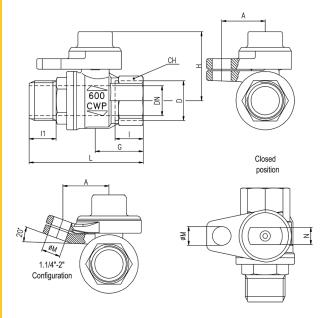
DN shows the nominal flow diameter. Actual flow diameter complies with full port DIN 3357 part 4.
