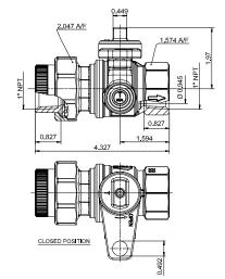
DN shows the nominal flow diameter. Actual flow diameter complies with full port DIN 3357 part 4.
