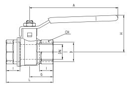
Part description Material Q.ty Unplated NPT body 1 CW617N 2 2 PTFE Seat Chrome plated ball 1 CW617N Unplated NPT end-cap 1 CW617N 5 Nickel plated stem O-ring design 1 CW617N 6 Geomet<sup>®</sup> nut 1 CB4FF 7 O-Ring 2 FPM Yellow PVC coated 8 1 DD11 Geomet<sup>®</sup> steel handle
