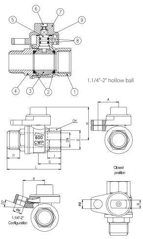
DN shows the nominal flow diameter. Actual flow diameter complies with full port DIN 3357 part 4.
