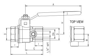
**Part description** Q.ty Material CW617N Unplated body 1 2 2 Seat PTFE 1 3 Chrome plated ball CW617N 4 Unplated end-cap 1 CW617N 5 Nickel plated stem O-ring design 1 CW617N 6 Geomet<sup>®</sup> nut 1 CB4FF 7 O-Ring 2 FPM Yellow PVC coated Geomet® steel 8 1 DD11 handle 9 Unplated plug 1 CW617N
