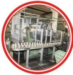
Automatic valve assembly and testing equipment 1/8" thru 4"
