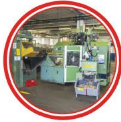
Transfer machines for forgings with automatic loaders
