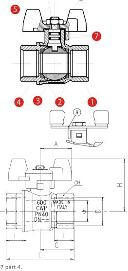
DN shows the nominal flow diameter. Actual flow diameter complies with full port DIN 3357 part 4. Ball valves are marked CE on body from 1 1/4" to 1 1/2": CE 0425 cat IIIB+D PS: 5 GAS TS1:-20°C TS2: +60°C
